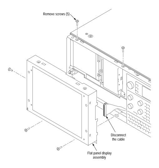
Figure 3: Flat panel display assembly removal
