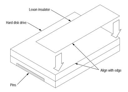
Figure 11: Applying the Lexan insulator
