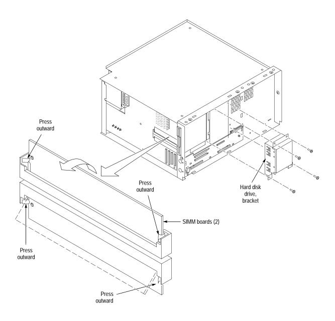
Figure 4: SIMM boards and hard disk drive replacement
