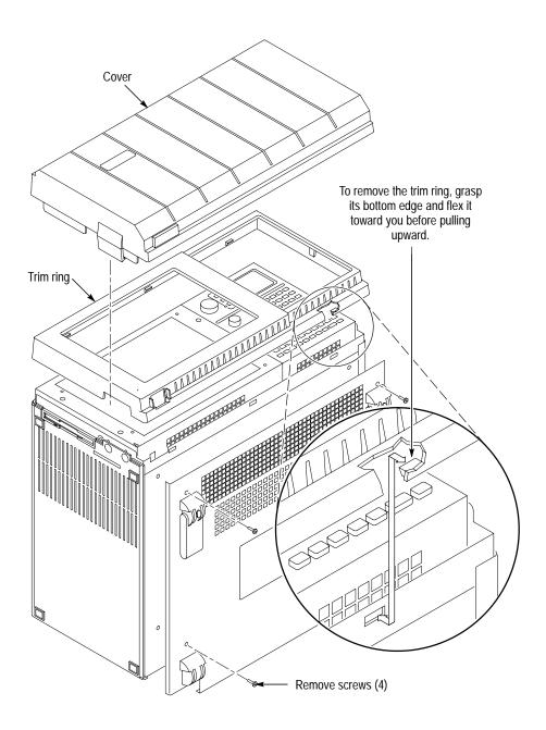
Figure 1: Front cover and trim ring removal
