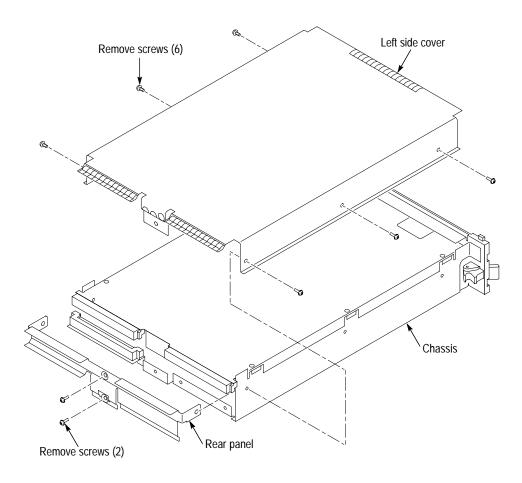
Figure 5: Left side cover and rear panel removal
