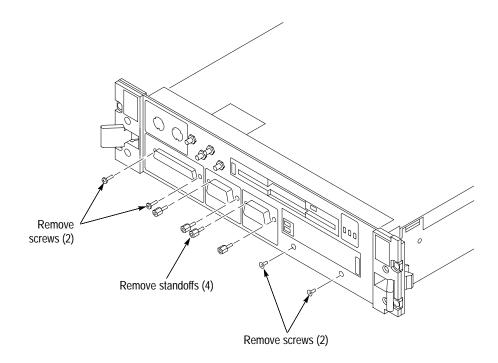
Figure 6: Front panel hardware removal
