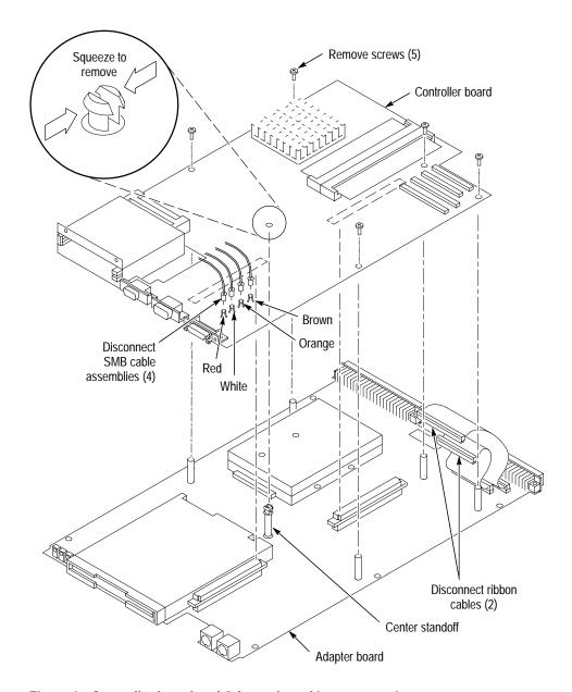
Figure 9: Controller board and Adapter board interconnection
