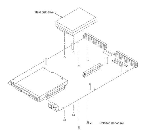
Figure 10: Hard disk drive removal
