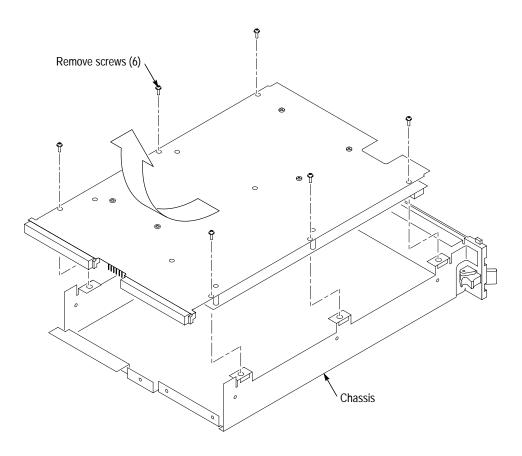
Figure 7: Subassembly removal
