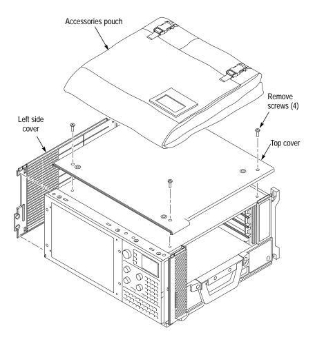
Figure 2: Pouch, top cover and left side cover removal
