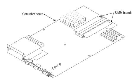
Figure 8: SIMM boards removal
